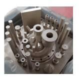
Small-scale combustion chamber and injector, ArianeGroup GmbH
